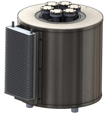
Oven with reactor and cooling system
